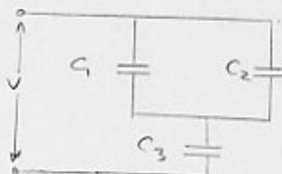
$$\frac{1}{C_{123}} = \frac{1}{C_{12}} + \frac{1}{C_3} = \frac{1}{17.3} + \frac{1}{4.5} = 0.280 \mu F^{-1}$$
