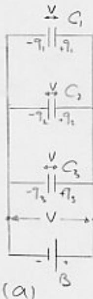
$$q = q_1 + q_2 + q_3 = (C_1 + C_2 + C_3)V$$
