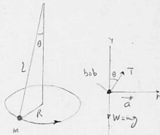
There must be a net force along the R axis providing the centrifugal acc.
