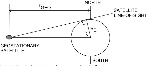
How high (in latitude) can a geostationary satellite view? The maximum northern latitude is given by
