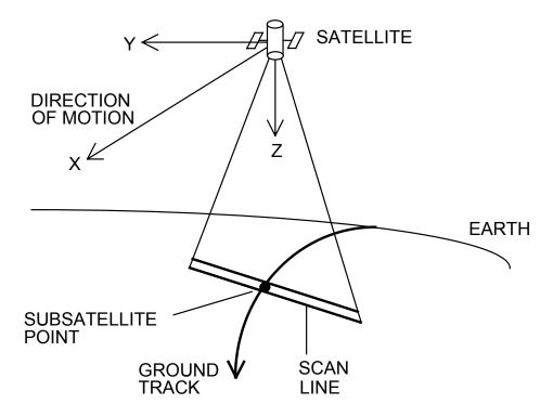
Three angles define the satellite orientation in this system:
