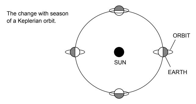
These orbits are simple as viewed from space, but complicated when seen from Earth because Earth rotates beneath the fixed orbit. This generally results in two daily passes of the satellite above any point on Earth: one as the orbit ascends and one as the orbit descends (usually one at day and one at night) with the time changing through the year.
