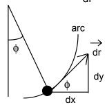
$$W = \int_{\phi=0}^{\phi=\varphi_o} \vec{F} \bullet d\vec{r} = \int_{r(0)}^{r(\varphi_o)} F \cos \phi dr = \int_{r(0)}^{r(\varphi_o)} (mg \tan \phi) \cos \phi dr$$
