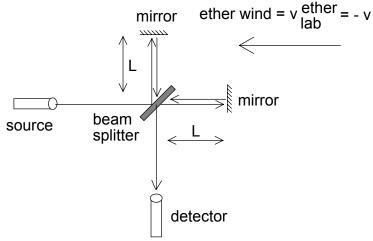
(A) First consider the round trip parallel to the motion (ether wind) and back.
