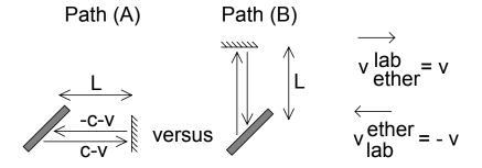
(B) Now consider the round trip perpendicular to the motion (ether wind) and back.
