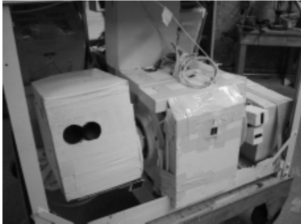
FIG. 6. Pointing system mounted in gondola frame in the flight configuration with the SPS instrument (left), pointing system housing (center), and sun sensors (right).
