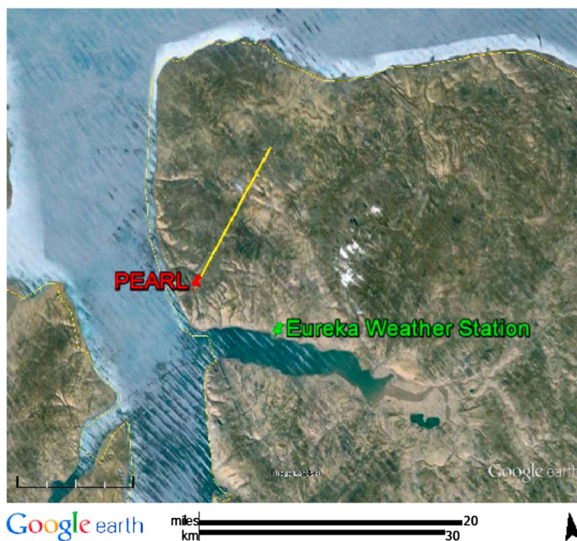
Figure 1. Locations of Eureka Weather Station and PEARL Ridge Lab (map data: Google earth). The yellow line (20 km in length) represents the viewing azimuth direction of MAX-DOAS measurements, which is 35° from true north.
