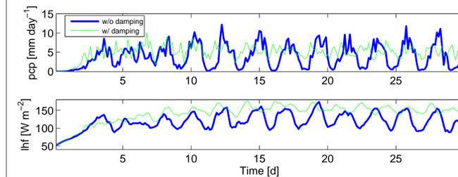
The impact of the resonant gravity waves on processes in the TTL is lessened by damping the velocity and temperature anomalies at the edges of the domain to their local mean value (accumulated with a ten day averaging timescale). The damping timescale is four hours at the edges of the domain and increases away from the edges of the domain as  $1/\cos(\pi x/L_x)^8$  and also increases in the boundary layer, so that the damping has negligible impact near the surface and in the convecting region.
