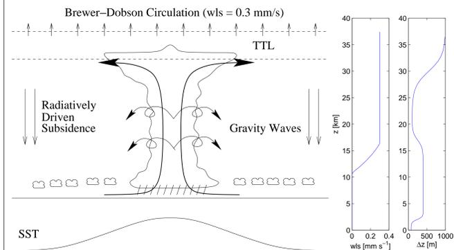
Domain:  $L_x \times L_z = 4096 \times 38$  km, with  $\Delta x = 2$  km and  $\Delta z = 75$ – $400$  m below a damping layer from 26–38 km.  $SST(x) = 299.15K - 2K \sin(2\pi x/L_x)$ . Simulations are run for 200 days, and averages/frequency distributions are computed from days 100 to 200.
