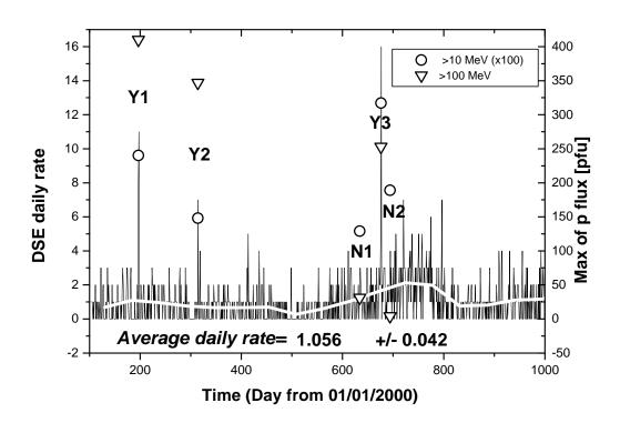
Fig. 5 Correlation between number of DSE during SPEs and the SPE proton fluence for E> 15 MeV ( in units of 10<sup>10</sup> particles/cm<sup>2</sup>). Y# and N# refer to SPRs identified in Table 1.
