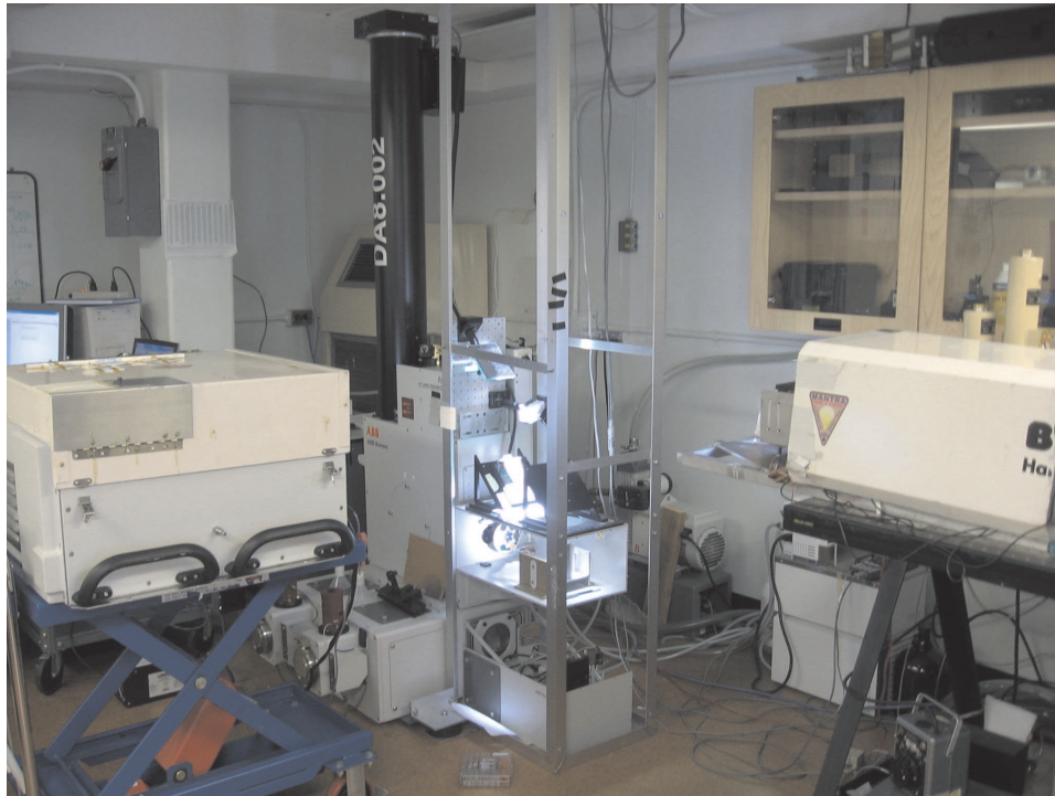
Figure 5.38: Photograph of the experimental setup. The PARIS-IR is on the left of the picture, the U of T FTS is on the right, and the TAO-FTS is located in the centre.
