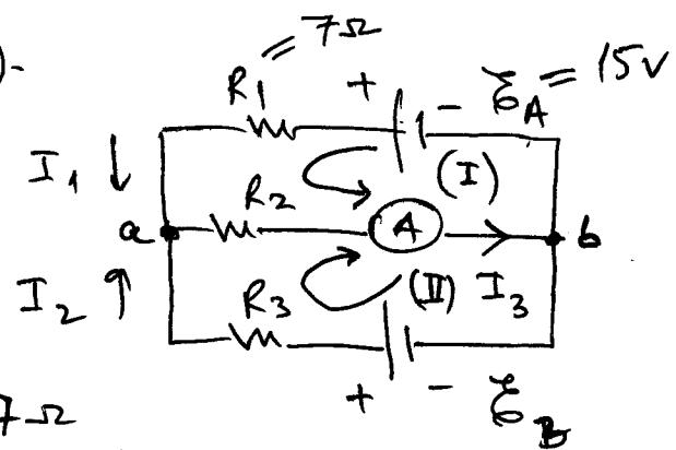
$$\left\{ \begin{array}{l} R_1 = 7 \Omega \\ R_2 = 5 \Omega \\ R_3 = 2 \Omega \\ E_A = 15V \end{array} \right.$$
