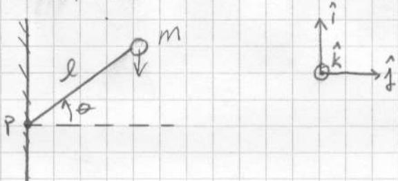
Recall that angular momentum is given by  $\bar{L} = \bar{r} \times \bar{p}$
