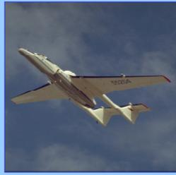
During several field campaigns the University of Frankfurt's "High Altitude Gas Analyzer" (HAGAR) measured  $N_2O$ ,  $CH_4$ ,  $CO_2$ , CFC-12, CFC-11, H-1211 and  $SF_6$  within the tropical UTLS region on board the M55 Geophysica high altitude aircraft. Ozone was obtained by the Fast Ozone Analyzer (FOZAN).
