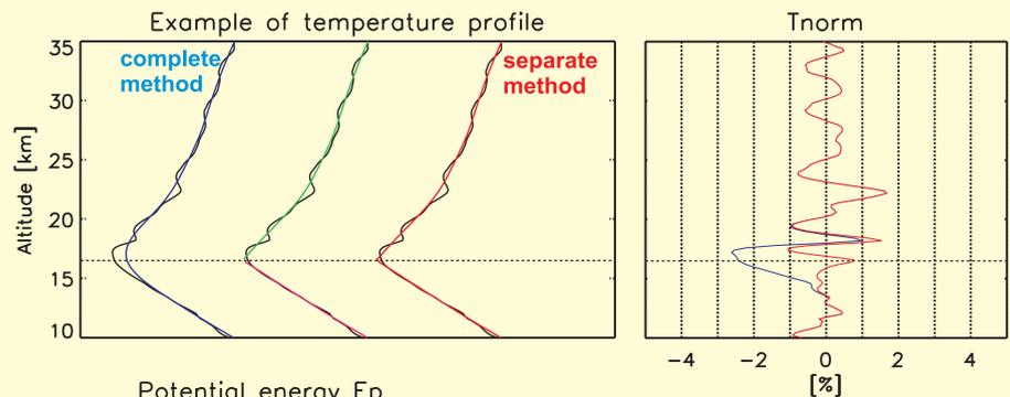
Fig. 3: Example for the determination of a temperature background profile with the complete and separate filtering method.
