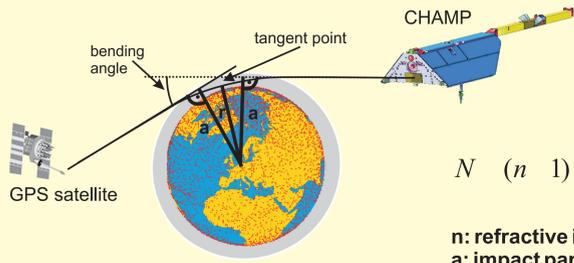
Fig. 1: GPS radio occultation principle.
