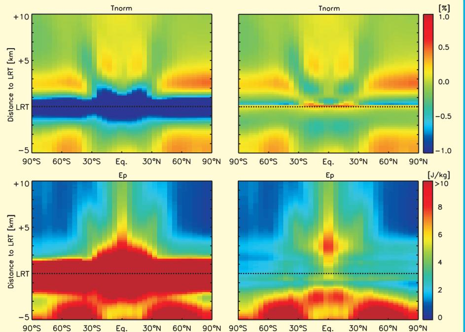
Fig. 5: Climatological normalized temperature (top) and potential energy (bottom) relative to the LRT for the complete (left) and separate (right) filtering method and the time interval from May 2001 to February 2008. The horizontal dashed line marks the lapse rate tropopause.
