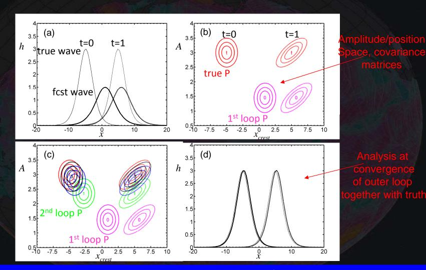
Example of effect of outer loop on analysis of solitary wave. Observations are of wave amplitude at every second grid point at the final time position of the wave.
