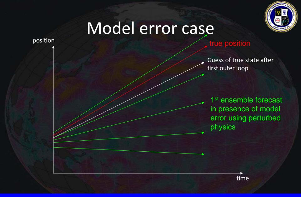
Initial ensemble is not centered on the truth. It has more spread than the ensemble of historical control/mean forecasts because each model has a different set of parameters. How can the outer loop be used to generate a covariance similar to that on the previous slide?
