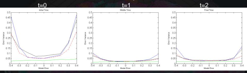
Variation of 0.1 in model error corresponds to a 1 sigma deviation of a parameter that affects propagation of solitary wave
