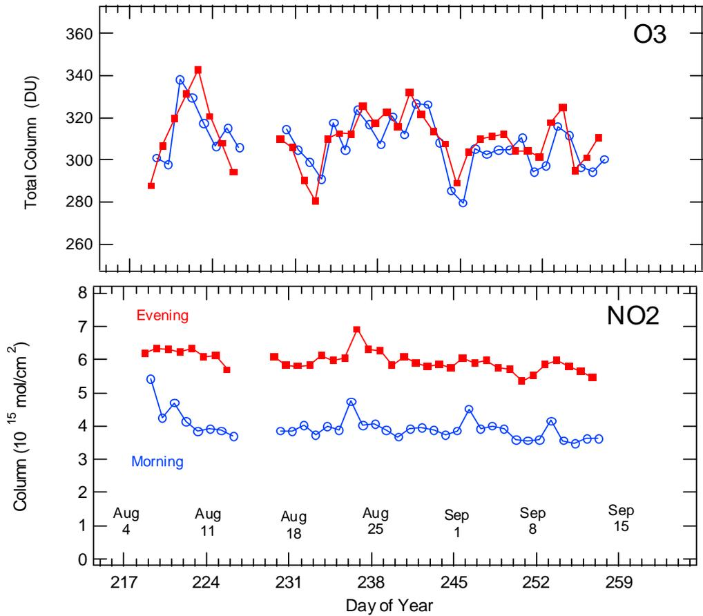
Figure 1: Time evolution in days of the ozone (top) and NO<sub>2</sub> (bottom) vertical column densities measured by the SAOZ ground-based spectrometer in Vanscoy during the MANTRA 2004 campaign. While ozone is variable between 280 and 340 DU, NO<sub>2</sub> was relatively stable with an average of  $5.96 \times 10^{15}$  molec.cm<sup>-2</sup> in the evening and  $3.96 \times 10^{15}$  molec.cm<sup>-2</sup> in the morning. Data provided by Florence Goutail.
