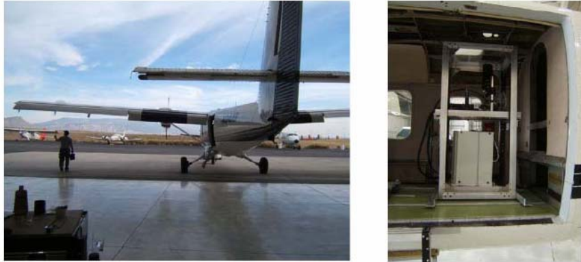
Figure 3. Photograph of the Twin Otter aircraft (left) and the new Phoenix Field Lidar (right) during installation on the Twin Otter at Grand Junction Colorado (base of Twin Otter Airborne Research).
