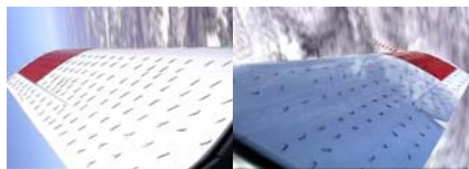
wing-flow visualisation post-transition to low- \alpha spin mode. \theta = -68.5^{\circ}
