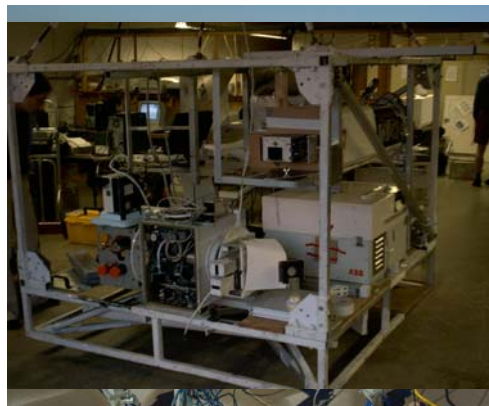
PARIS-IR on MANTRA 2004 gondola PARIS-IR in operation (with suntracker) during early stages of integration at Waterloo Atmospheric Observatory
