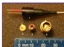
Fig. 2. Packaging VCSELs (VERTILAS, Germany): 1) laser is coupled with an optical fiber; 2) laser chip is mounted on a heat sink; 3) TO-46 package with AR coated optical window; 4) laser chip is mounted on a Peltier cooler.
