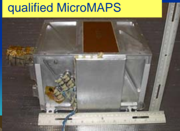
5 kg 3 gas channel space qualified MicroMAPS
