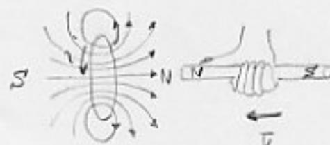
The induced current set up a mag. field that opposes the motion of magnet.
