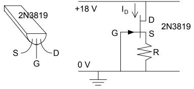
(2) Using the circuit in the figure below, with the same 2N3819 JFET, adjust  $R_S$  to make the drain current  $I_D = 0.5$  mA. Measure the gain of the circuit at 10 kHz and find the maximum undistorted output voltage. Verify that the gain of the circuit approximately agrees with the formula:
