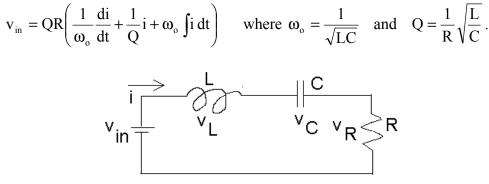
If  $v_{in}$  is sinusoidal, then the relation between  $v_{in}$  and i is given by  $v_{in} = R \left[ 1 + jQ \left( \frac{\omega}{\omega_o} - \frac{\omega_o}{\omega} \right) \right] i$
