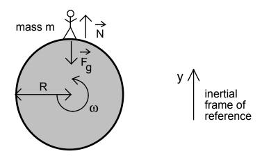
(a) There are two forces acting on the person: a normal force and the force of gravity, so  $\vec{F}_{net} = \vec{N} + \vec{F}_{net} = N\hat{j} - mg\hat{j}$
