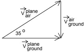
$\vec{V}_{air}^{plane}$  is the hypotenuse of a right angle triangle, so
