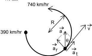
(a) In order to find the magnitude of the plane's acceleration midway through the turn, we first determine the tangential and radial components of the acceleration.
