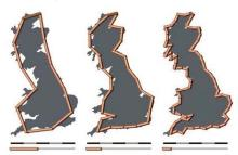
"The coastline of Britain as measured with measuring rods of 200 km, 100 km and 50 km in length. The resulting coastline is about 2350 km, 2775 km and 3425 km; the shorter the scale, the longer the measured length of the coast." ttp://upload.wikimedia.org/wikipedia/commons/2/20/Britain-fractal-coastline-combined.jpg
