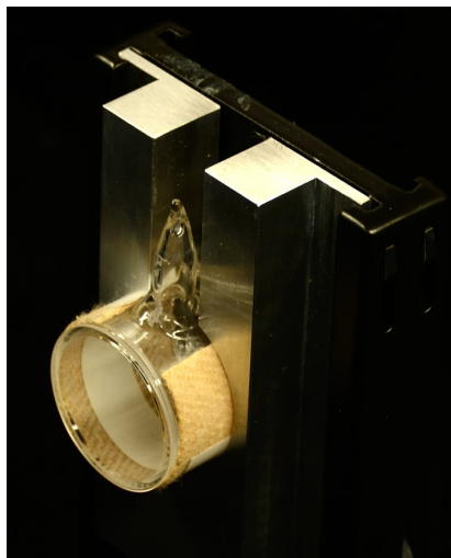
Figure 2.7: HBr cell #30 in its holder inside the PEARL Bruker IFS 125HR rear sample compartment.
