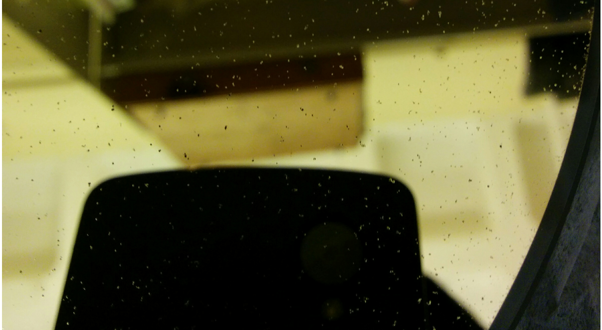
Figure A.2: D-mirror showing signs of coating degradation.
