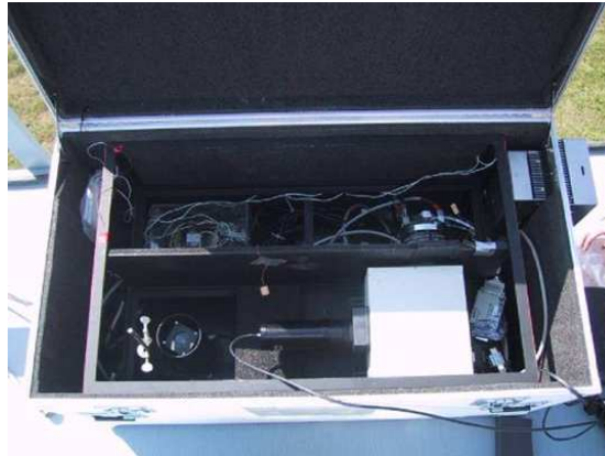
Figure 3.5: The UT GBS system assembled and located inside the second box for the MANTRA 2002 campaign.
