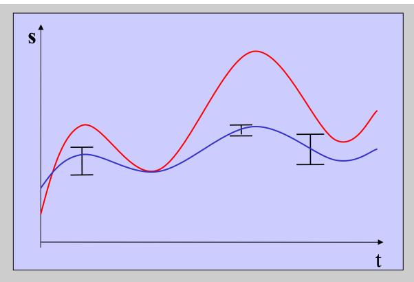
$$J(x) = \frac{1}{2} ((M(x) - d)^T C_d^{-1} (M(x) - d) + (x - p)^T C_p^{-1} (x - p))$$
