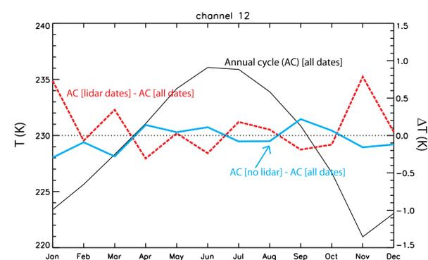
Figure 5 : NOAA-16 AMSU-A channel 12 annual cycle brightness temperature (in K; black), using all dates, and differences between annual cycle temperatures using only days with OHP lidar measurements (in K; red), or only dates without lidar measurements (in K; blue).
