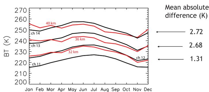
Figure 2: AMSU-A brightness temperature (K) annual cycle for different stratospheric channels (black), and temperature (K) annual cycle for selected altitudes of OHP lidar measurements (red).
