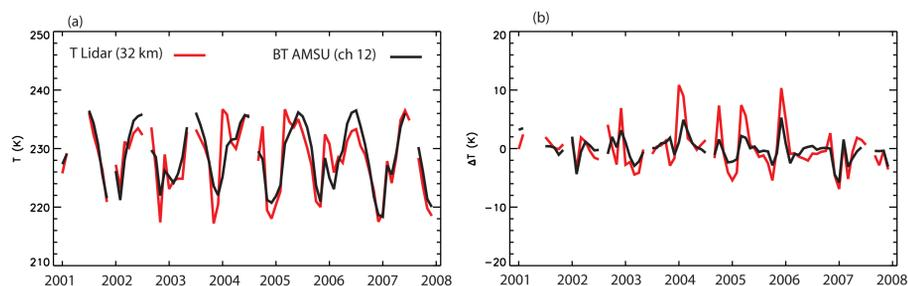
Figure 3: (a) Time series and (b) time series with annual cycle removed, of temperature at 32 km measured by lidar and brightness temperature from AMSU-A channel 12.
